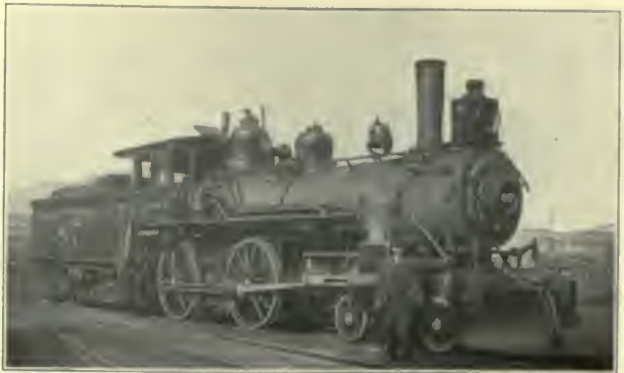
FIG. 381. LOCOMOTIVES. Passenger Locomotive of the American Type. Atchison, Topeka & Santa Fe Railway.
